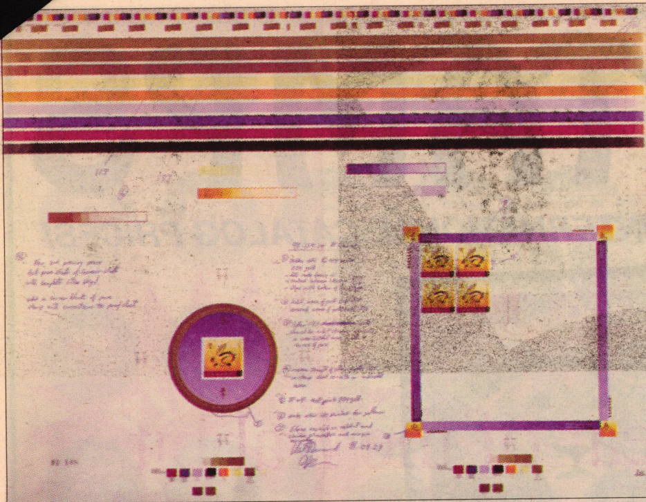
Figures 3: First proving proof sheet. This is where the proof sheet is marked up for color corrections to stamps and souvenir sheets. The stamp is proved on a block of four within the complete pane border.
